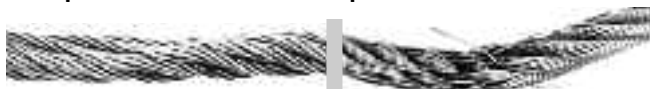
Crushing. Because of loose winding on drum, rope was pulled in between underlying wraps and crushed out of shape.
